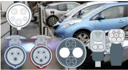
Figur 42 - Different technical forms of electric car charging contacts. Source: https://fdel.dk/guides/charge
